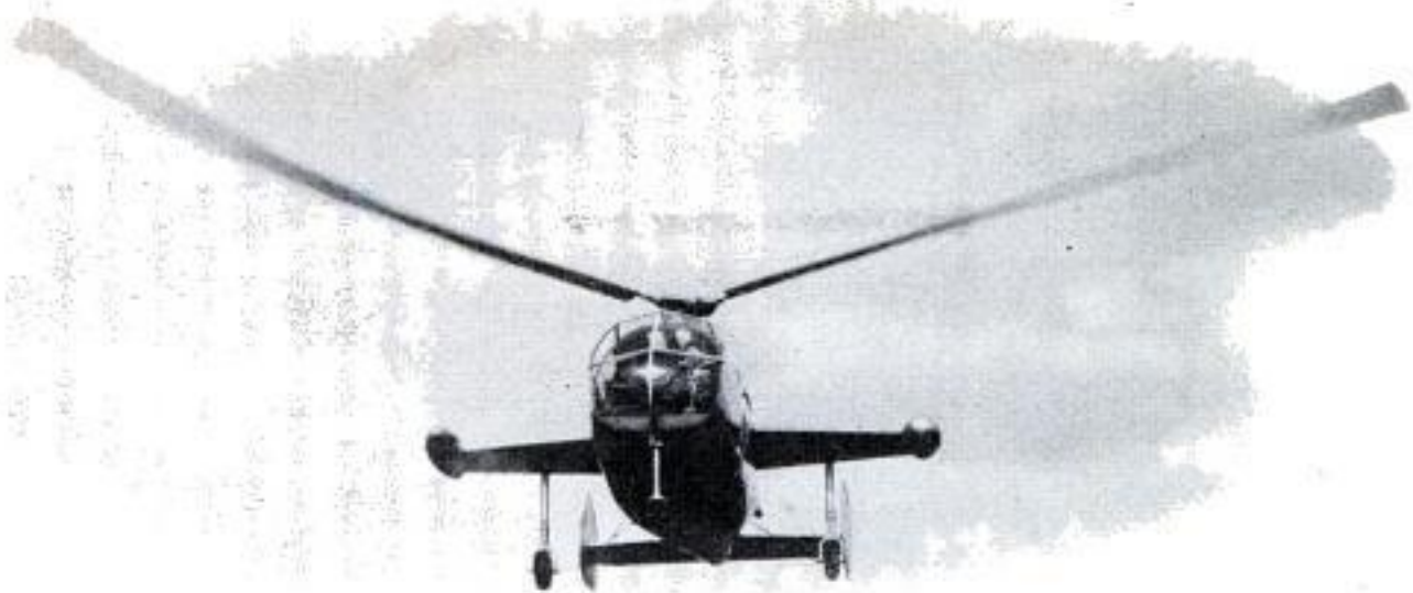
Flying Magazine photo Flying prototype of British Fairey Gyrodyne has two forward propellers on tips of stub wings and a three-bladed rotor
